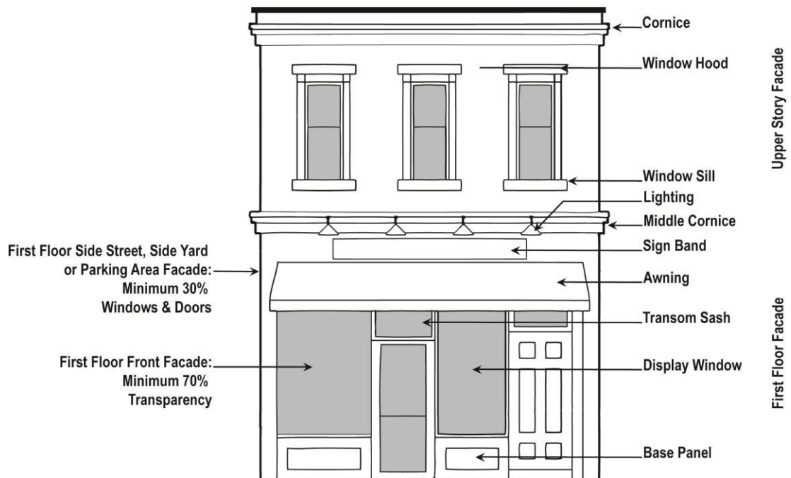
Figure 9-1. Transparency and Building Façade Features
